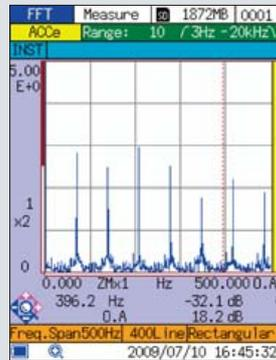
When diagnosing a bearing fault, it is necessary to know the repeat cycle of the impact waveform. This can be achieved by envelope processing, using the principle illustrated below.
