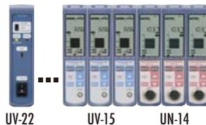
**Configure a measurement system for up to 16 channels by linking the Sound Level Meter Unit UN-14 and Vibration Level Meter Unit UV-15. Each unit has its own display showing settings, measurement values, and a bar graph indication. Adding the Interface Unit UV-22 allows connection to a computer for control of settings and operation and transfer of measurement data.**
