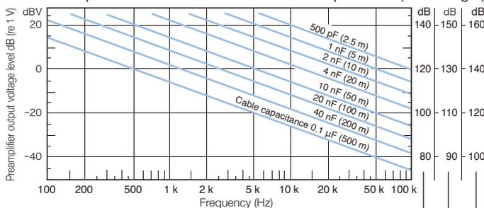
Measured sound pressure level at microphone sensitivity level -26 dB (re 1 V/Pa)
