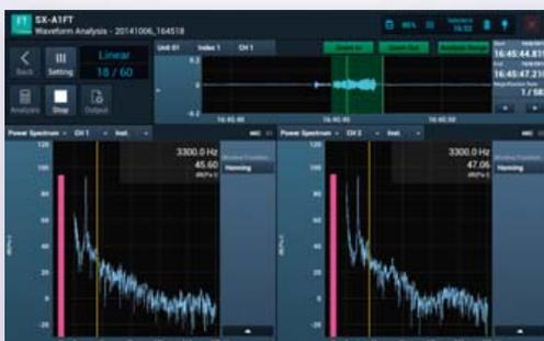
**RIONOTE** is combining the newest quality, ease of use and economical sense, which can be configured to up to 16 channels anywhere wireless. The Main Control Unit is program of your choice. All on a large color screen, both programs and hardware for this mea
