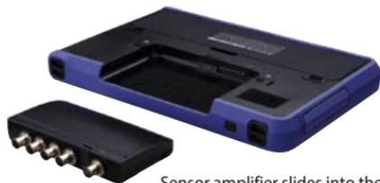
Sensor amplifier slides into the underside of main unit
